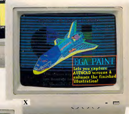
CC-1422 Dot pitch 0.31mm Reso. 720 x 350 Horiz. freq: 15.75KHz, 21.85KHz EGA compatible Nonglare CRT
