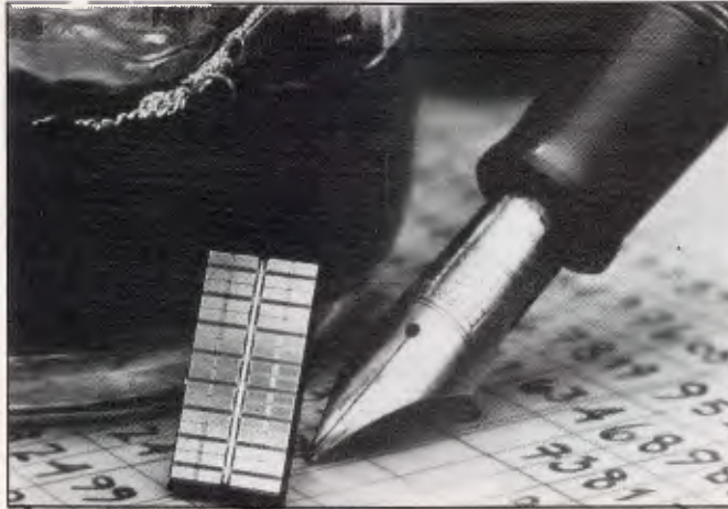
This is a four megabit chip which IBM claims it is able to fabricate on production lines currently used to produce one million bit chips. It has fast access (65 nanoseconds) and can store the equivalent of 400 pages of double-spaced typewritten text.
