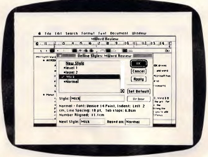
The Style Editor allows the user to define styles in terms of fonts, and so on. Editing a style effects a change everywhere the style is used
