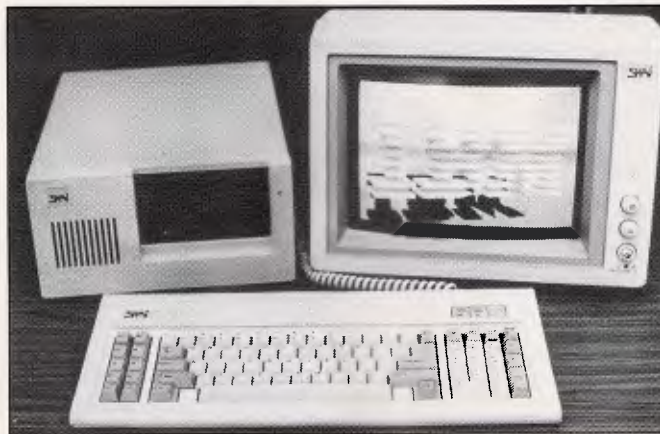
This little box contains an 80286 running at 10Mhz with zero wait-states. Which means it's pretty fast. Called the Pro-AT, the machine is from Skai and is sold by Porchester Computers, tel: (03) 537 2722.
