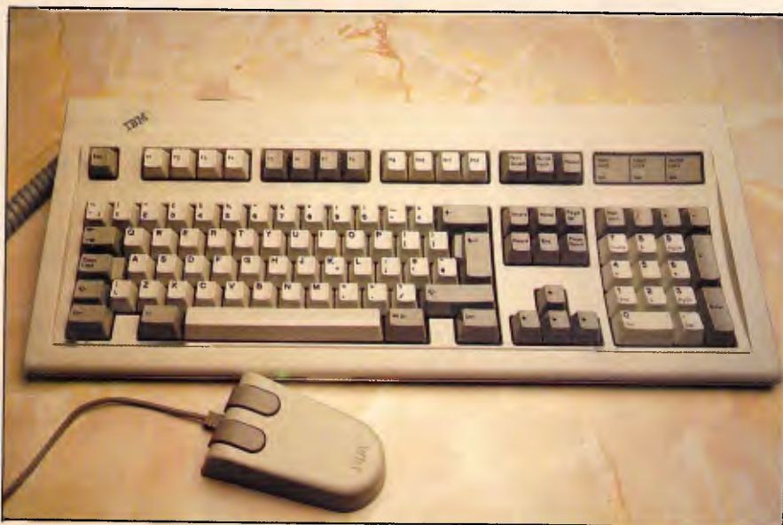
Reinforcing the AT/E as the standard PC keyboard, the 102-key unit includes a separate cursor and numeric pad — and twelve function keys seem to be the new gospel. The stylish mouse is a standard item
