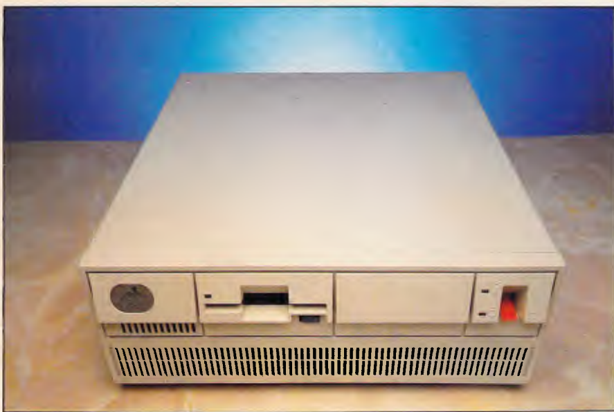
The new machines lack the bulk of previous PCs and the 3.5in disk drive may now be here to stay. The mains switch — a clumsy affair — has migrated to the front while the keyboard lock is now on the back
