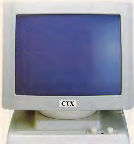
CC-1400 14" Dual Frequency Display Monitor Amber & Green * Horizontal frequency — 18.432KHz/15.75KHz * Vertical frequency — 50Hz/60Hz * Video response — 20MHz (-3dB) * Resolution — Over 1000 lines at center
