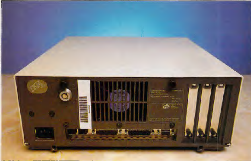
All the standard ports run off the motherboard, freeing slots for further expansion. From left to right: keyboard, mouse, bi-directional Centronics, RS232C and video out. The centrally-mounted fan is almost noiseless
